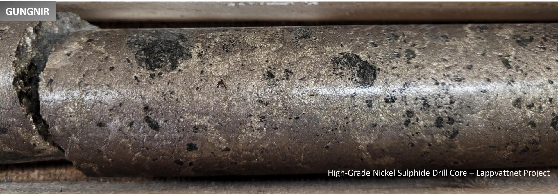
High-Grade Nickel Sulphide Drill Core – Lappvatnet Project
