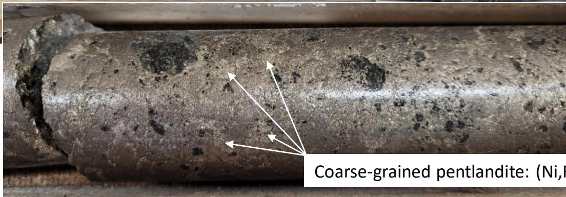
Coarse-grained pentlandite:  $(\text{Ni}, \text{Fe})_9\text{S}_8$
