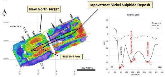
Slingram survey results. Strongest conductors are in red. Western half of the survey employed a 60-metre coil configuration and a 40-metre coil configuration was used for eastern part of the survey block. The larger discordant red anomaly in the easternmost part of the survey is likely resulting from conductive soils.
