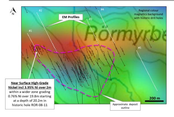
The survey will be completed by Geovista AB, from Lulea, Sweden using WalkTEM equipment from Guideline Geo. The instrument is a light-weight time-domain system with results expected to define the properties, geometry and depth extent of conductive bodies much better compared to a traditional Slingram system. Results of the survey will assist positioning of future drill holes.
