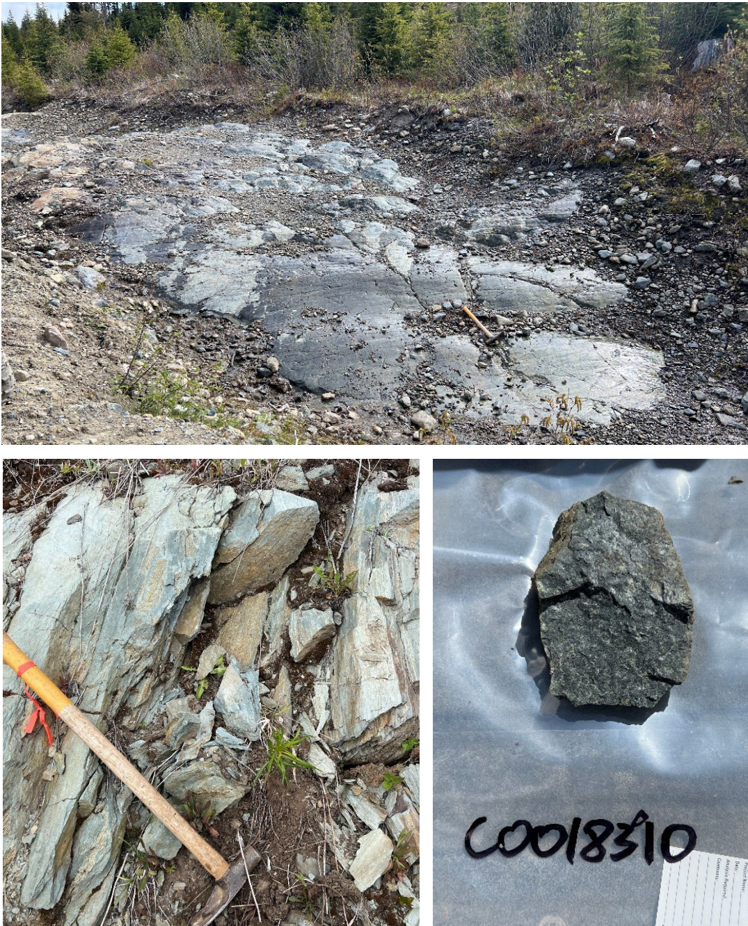
Figure 12-1: Site visit photos. Top – JHQNS001 glacial striations on roadside ultramafic outcrop. Bottom left – pale grey silicified metasediments Bottom right – ultramafic 2100 ppm Ni
